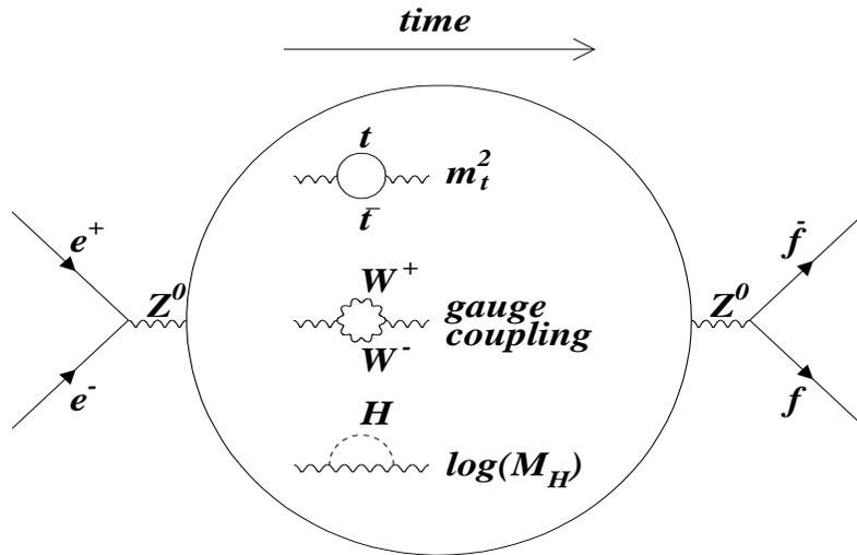
**Fig.1:** Diagramme representing the most frequent process occurring in  $e^+e^-$  annihilations at LEP, corrected for the dominant quantum fluctuations affecting the propagation of the  $Z^0$  boson: virtual pair of top-antitop ( $t\bar{t}$ ) quarks or of  $W^+W^-$  bosons, and virtual Higgs boson.
